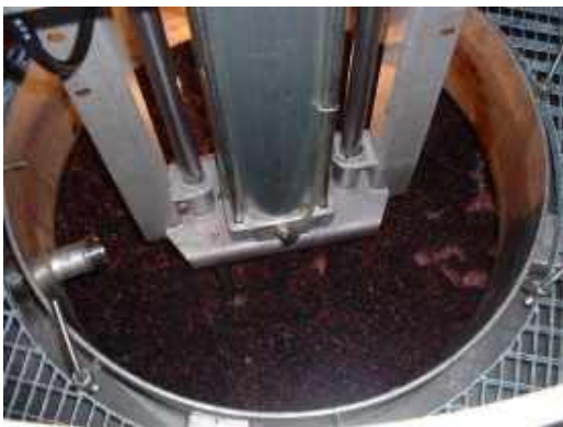
At left: a state-of-the-art "robo-pigeur" which thoroughly mixes the solids with the juice to attain full extraction of color and flavor. At right: all the wines ferment in stainless-steel tanks to ensure the freshest and purest wines.
